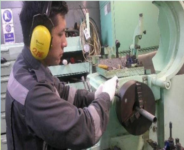
1. Tight chuck with material
